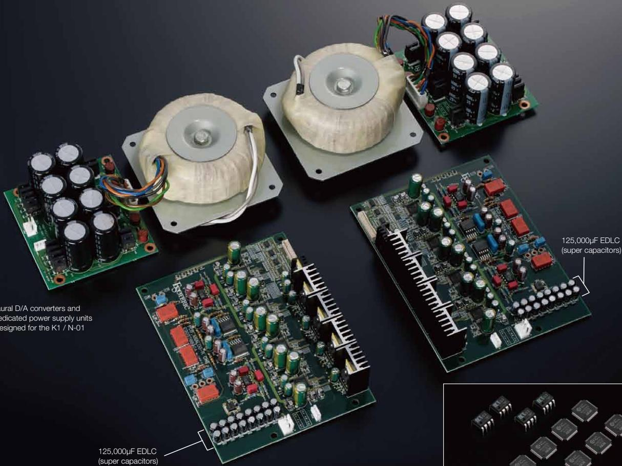
Dual monaural D/A converters and channel-dedicated power supply units specially designed for the K1 / N-01
